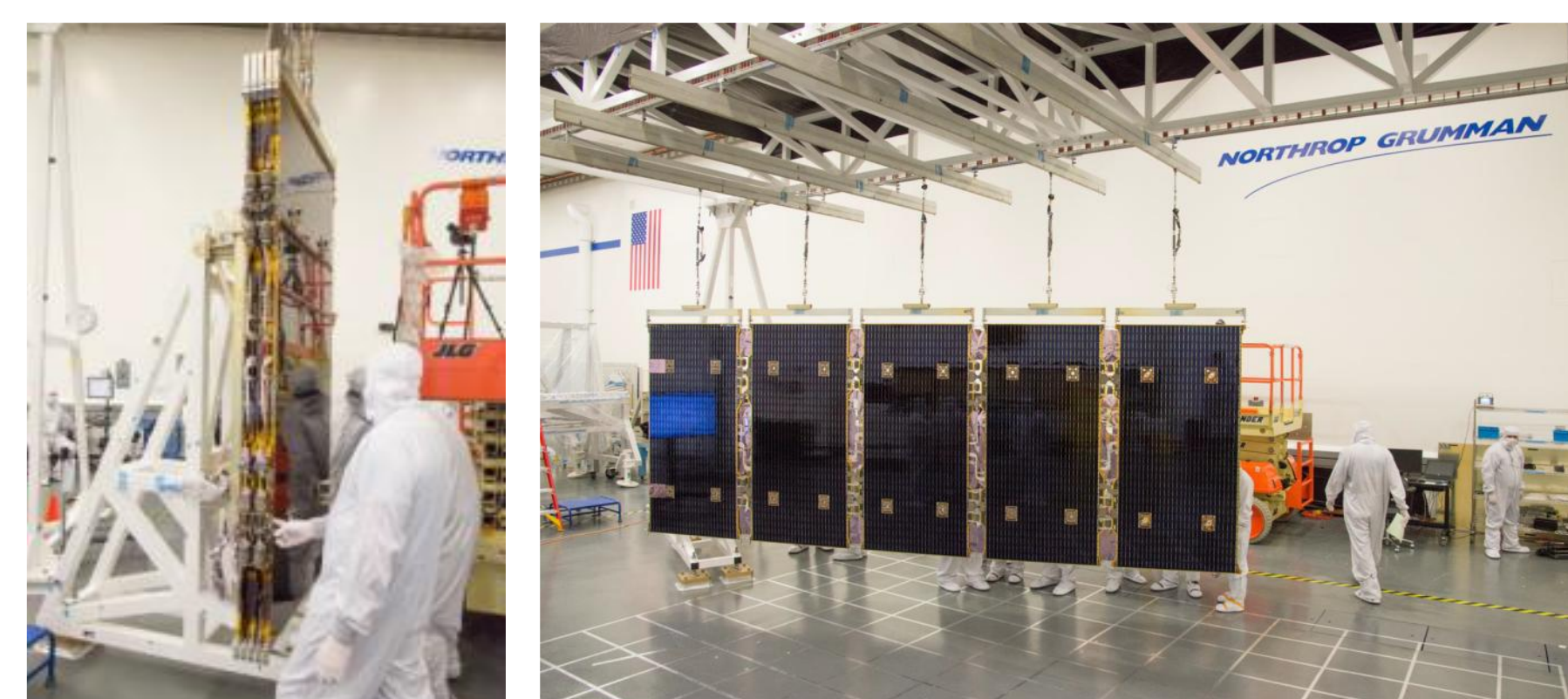
Solar Array Deployment Testing – Panel Unfolding
