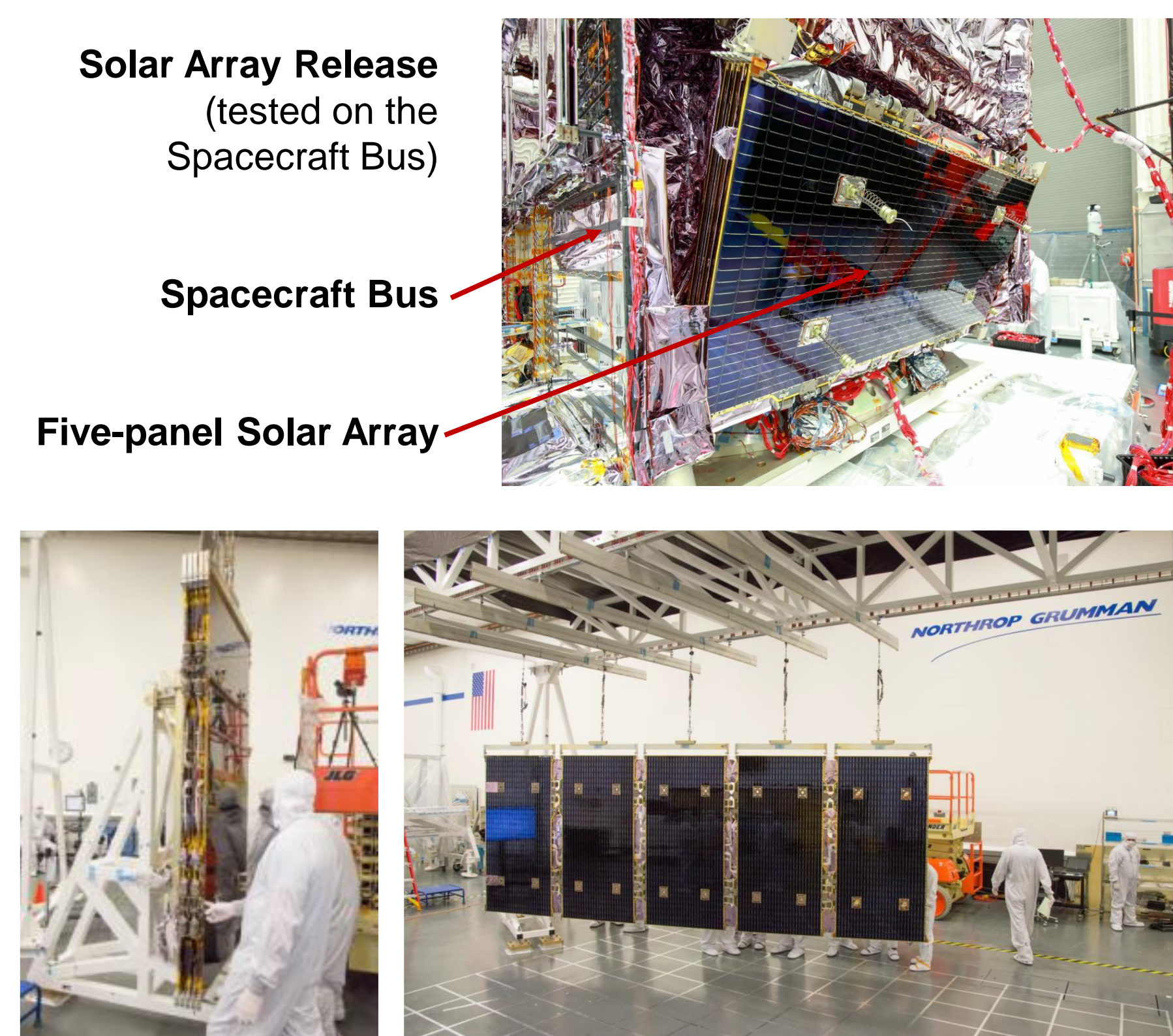
Solar Array Deployment Testing – Panel Unfolding
