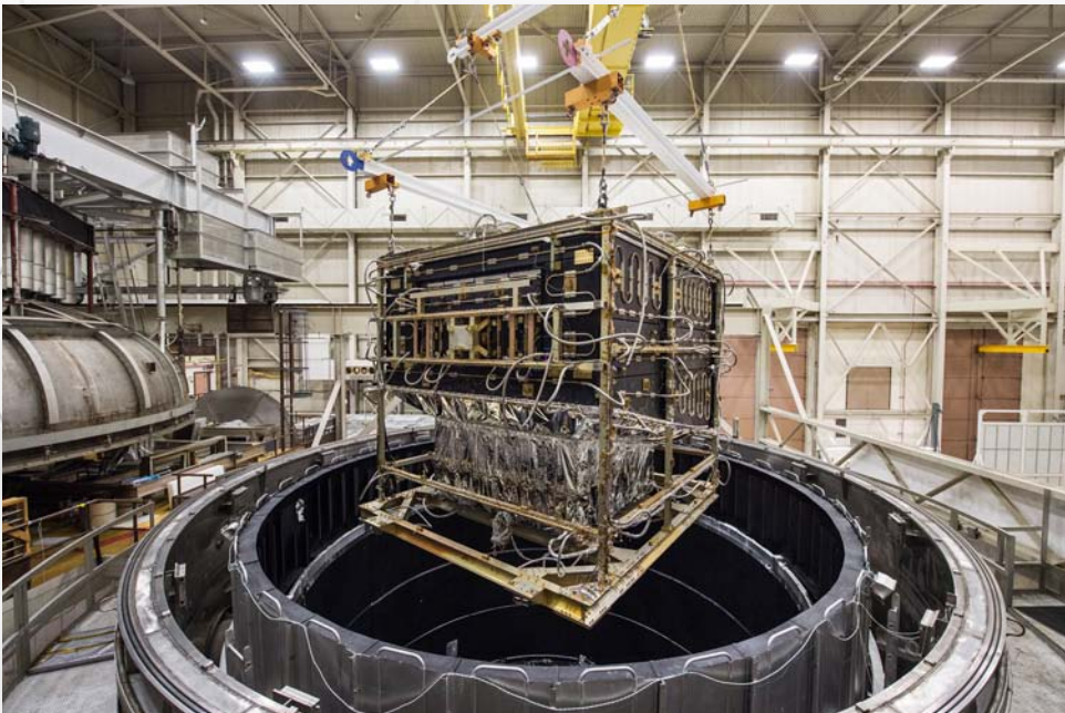
Figure 3. The Core2 test article being removed from NASA/Goddard's Space Environment Simulator (SES) following testing. When installed in the chamber, there were only 8 inches of vertical clearance with the chamber roof.
