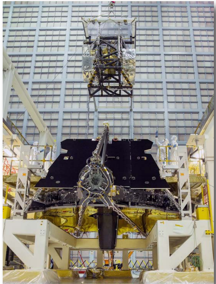
Figure 4. The JWST science instruments are lowered into position using a crane. The primary mirror segments can be seen facing the floor for this installation. A video of the installation process can be downloaded at http://svs.gsfc.nasa.gov/12273 .
